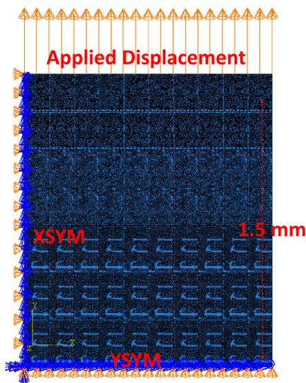
Figure 2- Boundary condition and loading
